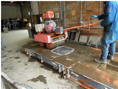
Fig. 26 – Preparation of Asphalt Concrete Beams
