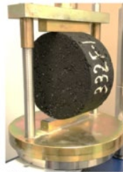
Figure 1 – IDEAL-CT test frame (left) and loading jig (right)
