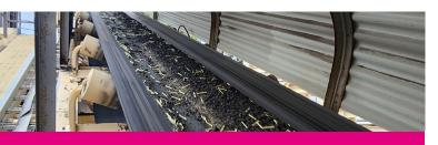
which introduced the low dose of fibre (106g/T) in a very consistent manner into the Astec Double Drum asphalt plant via the RAP conveyor.
